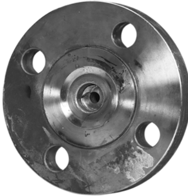
Fig. 3-36: Vibration crack corrosion example of a flange/thermowell connection. The crack started at the beginning of the threads on the process side.
