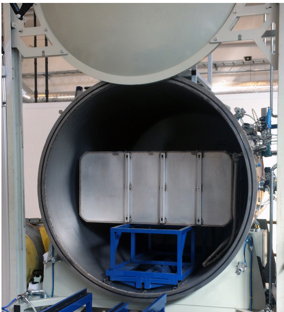
CCV AirPlus at gas tightness test
